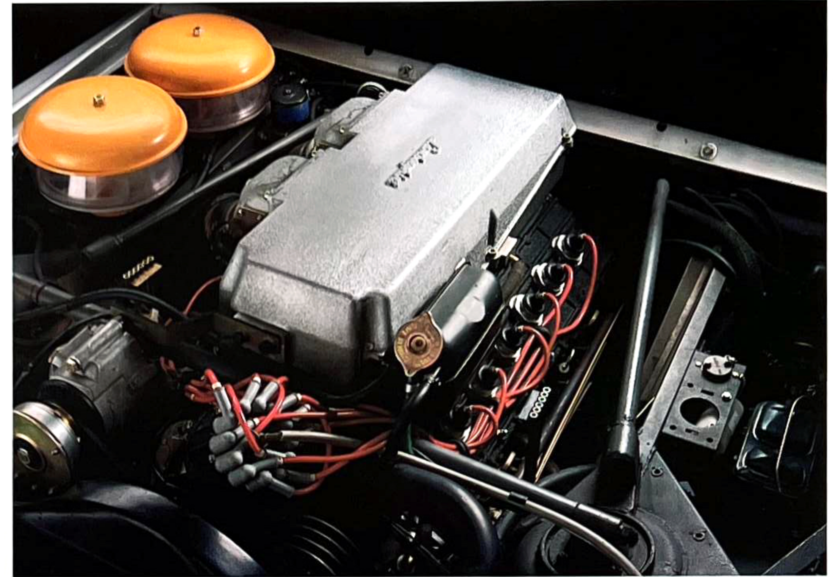
The LM002 standard 48-valve V-12 engine produces 455 hp @ 7,000 rpm.
